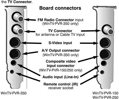
The S-Video/composite video input can be used to bring video from a VCR, camcorder, camera, DVD player or satellite TV receiver. On the WinTV-PVR-350, if your video device uses composite video instead of S-Video, use the supplied Composite to S-Video adapter. Plug your composite video connector (normally this is yellow) into one end of the Composite to S-Video adapter and the other end into the S-Video input on WinTV-PVR-350.
