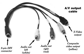
3. The A/V cable has Audio out left (white) and a Audio out right (red) jack. Connect these to the audio input jacks on your TV set (not supplied).
